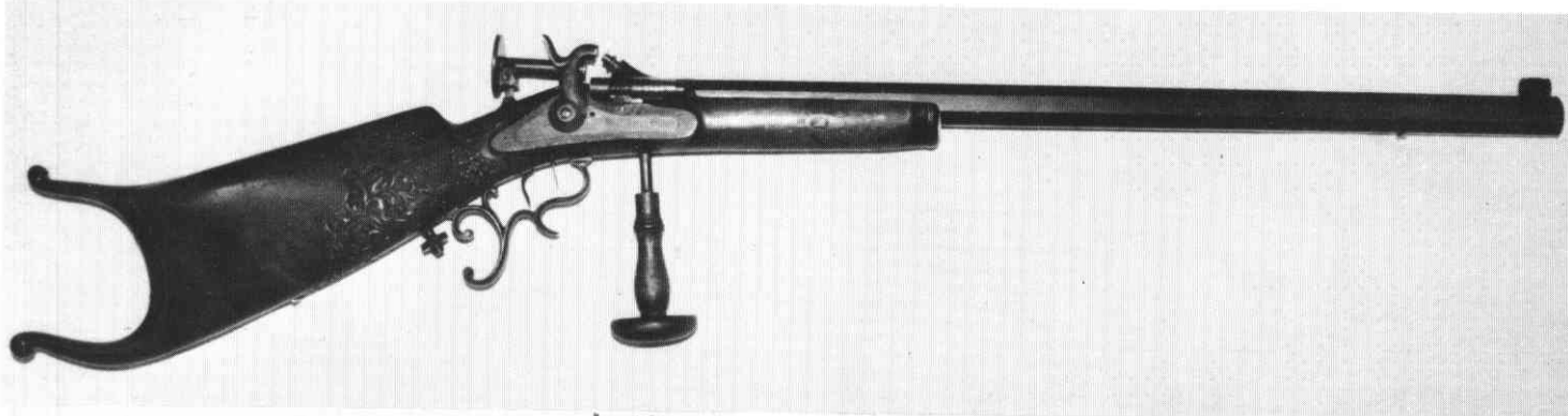
• Solid buttplate, large trigger guard screw; note shape of trigger guard; note applied thumb rest ("Daumenkanzel" - Thumb pulpit); stock heavily carved on both sides.
