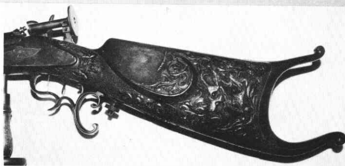
• Altered to centerfire. Only Meunier known that has been so altered: note large hammer, first model characteristics, carved deer head on left side of stock.
