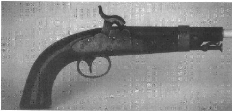
Model 1842 N.P. Ames, showing the rounded, flat, lockplate that was standard production after the first three hundred.
