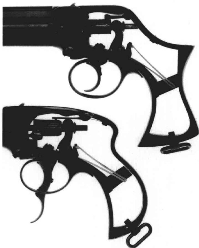
FIGURE 8. Interior views of Thorn patent pistols. Upper: Two barrel small frame holster pistol (.476 Rev., serial no. 8099). Lower: Four barrel large frame holster pistol (.476 Rev., serial no. 8342).
