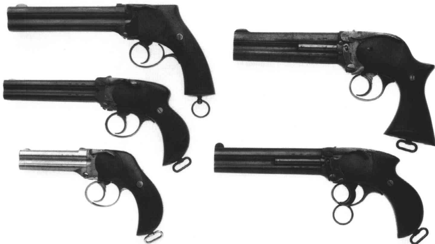
FIGURE 1. Examples of the basic model types. Left, four barrel pistols, top to bottom: large frame holster pistol (.455 Rev., serial no. 7205); small frame holster pistol (.380 Long, serial no. 8186); small frame pocket pistol (special order .380 Long, serial no. 7381). Right, two barrel pistols, top to bottom: large frame holster pistol (.577 c.f. for special order 1½ inch cartridge case, serial no. 8407); small frame holster pistol (.476 Rev., serial no. 8042, with ring type cocking trigger).
