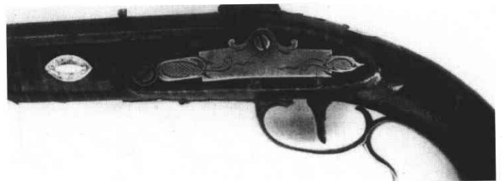
19. The A. Alloway pistol sideplate is typical of York County rifle sideplate design.
