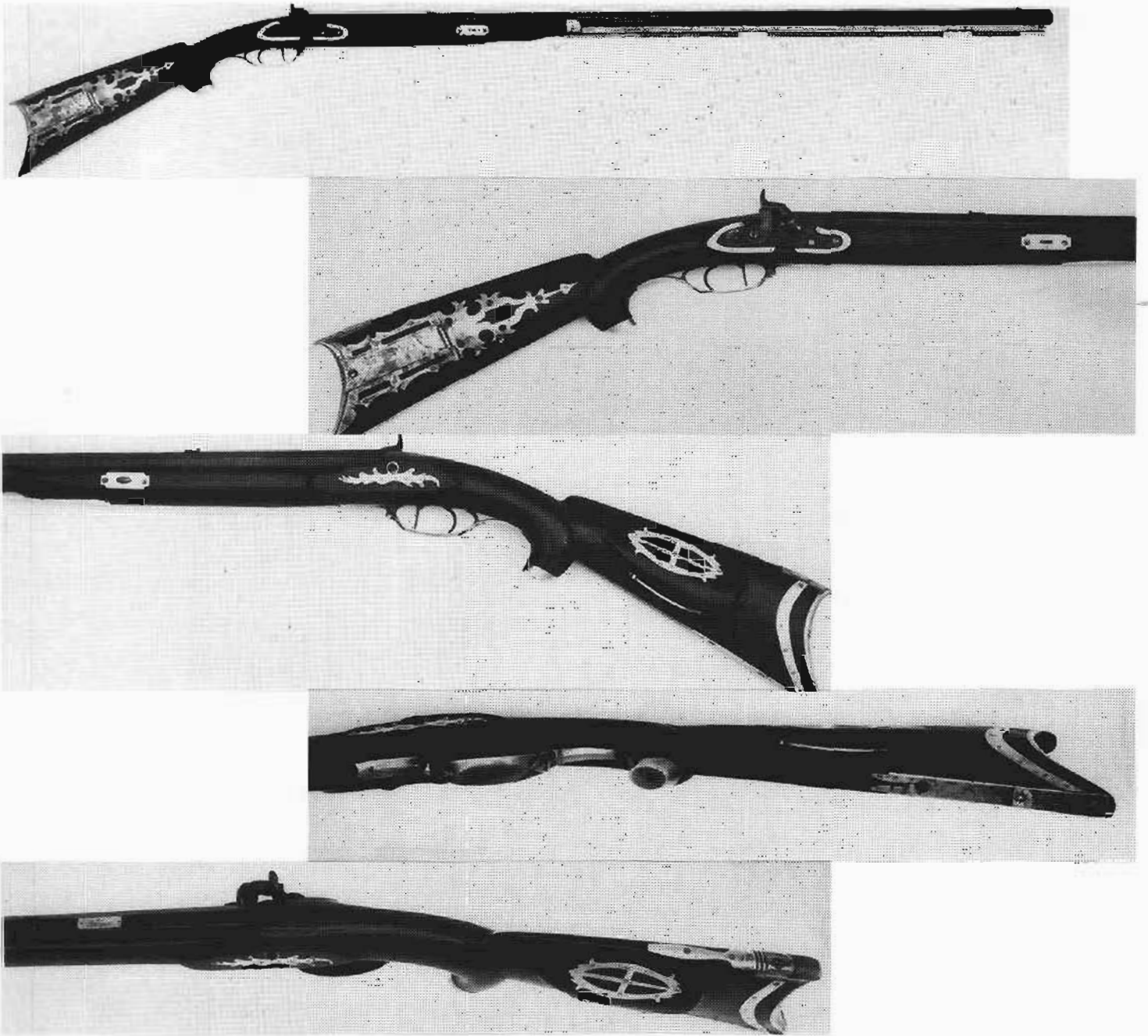
The "Pistol-Grip" longrifle. Ray McKnight collection. Half-stock of walnut, brass hardware, silver inlays, 38" barrel. Photos courtesy of Charles Semmer.
