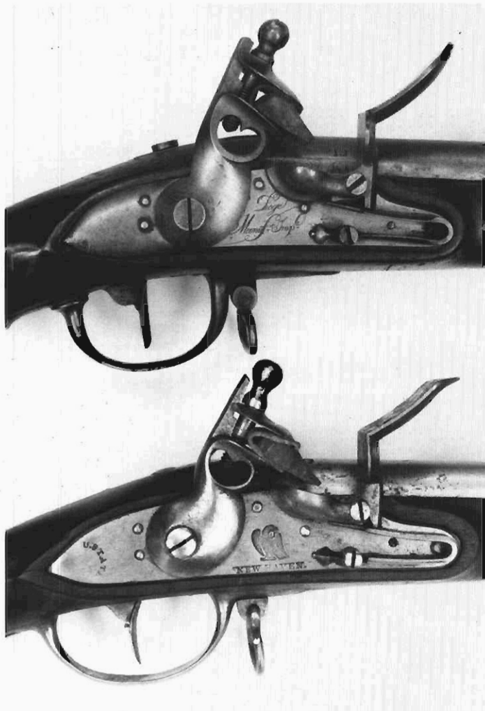
Figure 16. French Model 1777 improved an IX (top) and Whitney 1801 improved Model 1798 (lower) locks.
