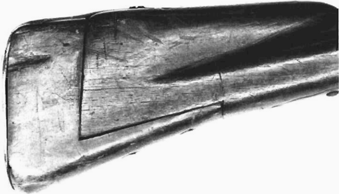
A butt from another musket had to be spliced onto the butt of this French musket.
