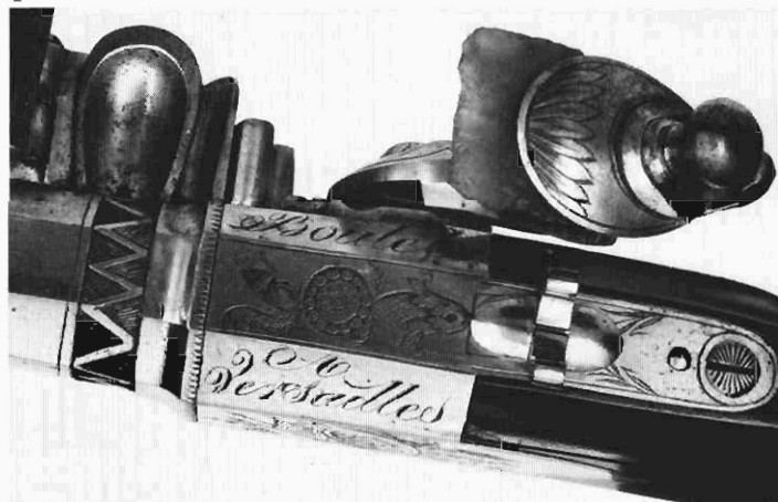
View of the top flat of the frame and signature panels of the pistol. Note the notched sliding safety which serves as a rear sight.
