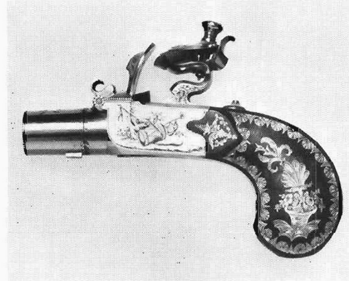
Smooth bore pocket pistol with screw-off barrel. Rosewood stock with silver inlaid engraved borders and motifs. Metropolitan Museum of Art.
