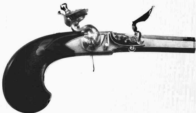
One of the pair of side hammer box lock pistols shown above. The roller on the frizzen spring may have been introduced by Boutet, based on British duellers which he may have seen.
