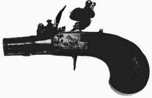
Box-lock, turn-off smooth bore pocket pistol, barrel engraved "LePage A Paris". Circa 1810.
