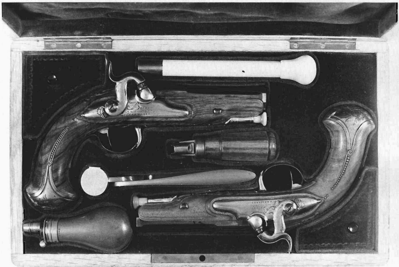
Early pre-Revolutionary pocket pistols by Nicholas Noël Boutet, circa 1788-1789, Louis XVI reign. Converted to percussion about 1825 and cased. Lockplates engraved "Boutet/Arq re Ord re Du Roi/Versailles". Barrels engraved "Boutet Versailles". 7 1/2 inches long, .57 calibre, multi-groove rifling. Author's collection.
