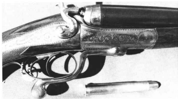
Locks of an I. Hollis & Sons, London, Double Rifle, caliber .500/.450 Nitro Express, shown with its cartridge.
