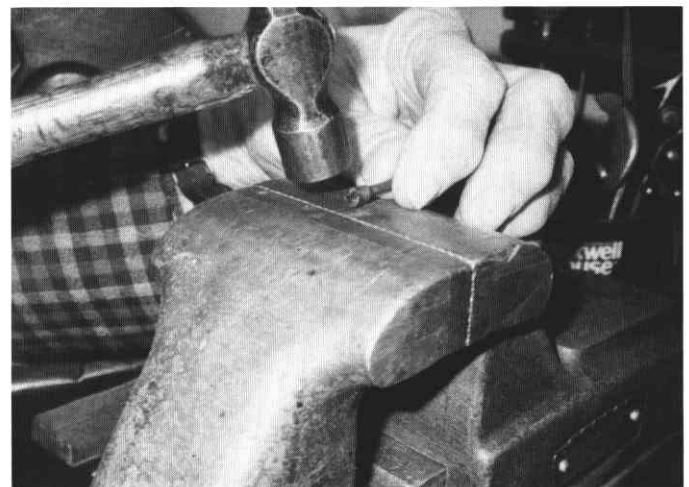
Two badly defaced screws in the pin stock to support the head.
