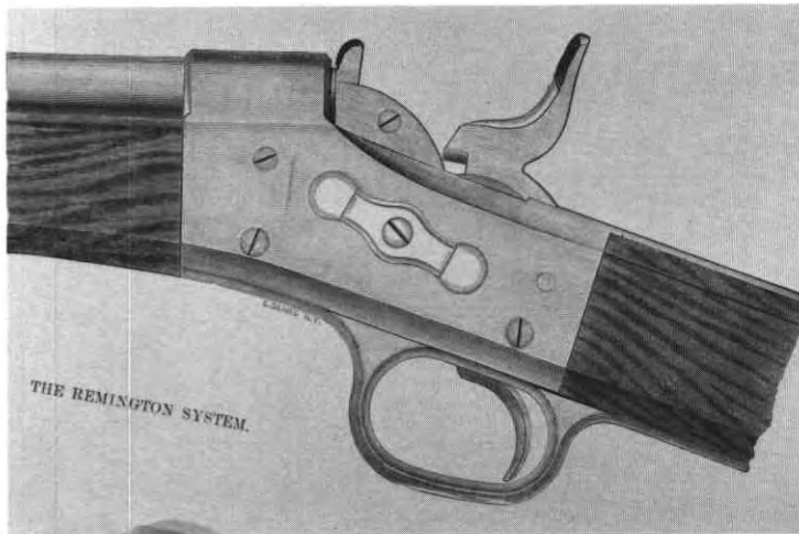
The Remington Rolling Block Action.
