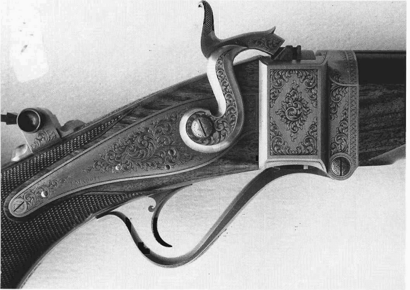
Model 1877 Sharps .45-2.6 inch caliber. Action and lock handmade and all metal parts by Madole except barrel. This, he contoured to include Rigby style flats.
