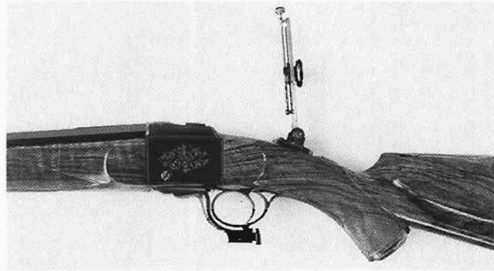
Alexander Henry modification of Ruger No. 1, in .45-70 caliber with perfect mating of wood with metal. Please note the quality of metal work in the fit and style of push button lever and sights.
