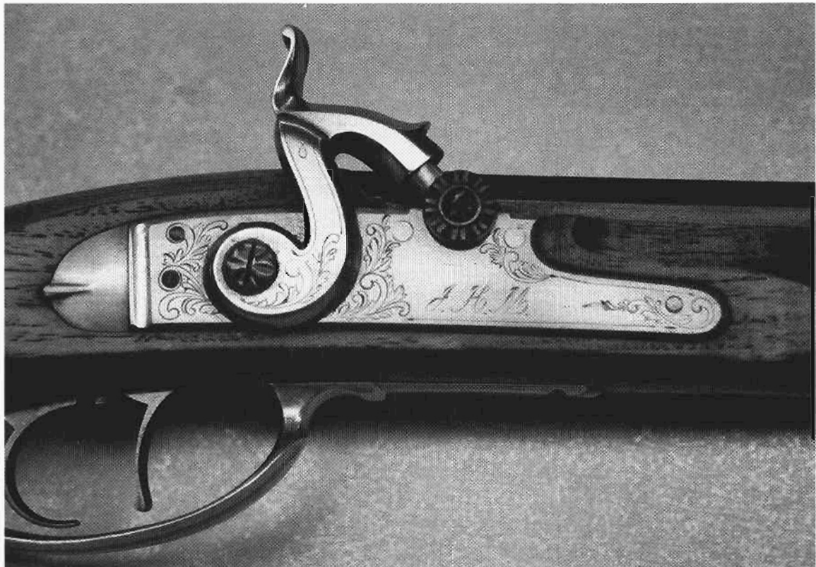
Detailed views of the muzzle loading rifle, showing handmade set triggers, lock, and the type engraving correct for an arm of this vintage.
