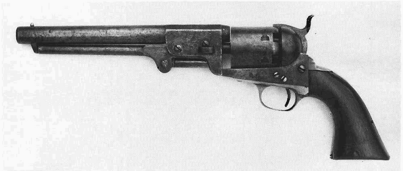
Leech & Rigdon revolver serial number 52. Note the longer barrel type, and that the brass portions have pitting-like casting flaws. No company markings are present on the barrel top flat. Author's collection.
