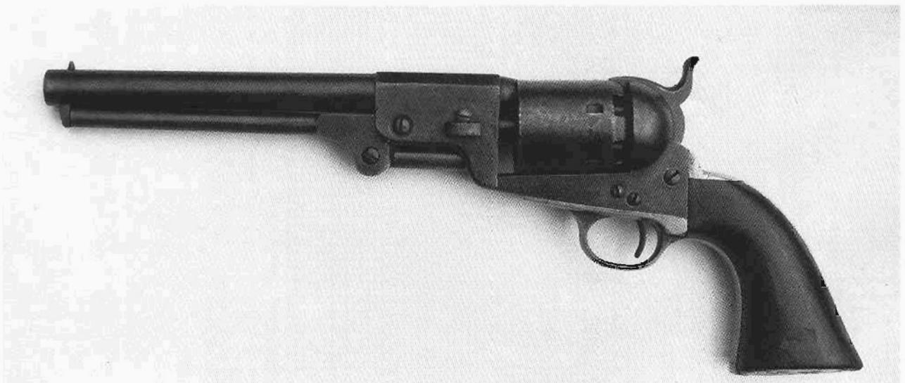
Leech & Rigdon revolver number 59. The company name stamping is the small sized die. The loading lever screw is serialized.
