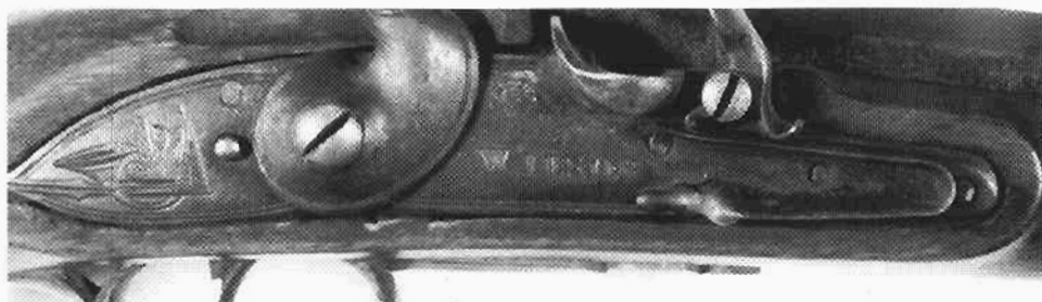
Figure 23a. Lock area of the Nock stocked Wilson Cypher gun. The slightly convex lockplate is 6 1/8" long and 1" wide at the fence.
