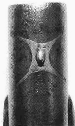
Figure 31. "Spider" front sight on the Grice gun. The splayed legs are inlaid into the metal of the barrel.
