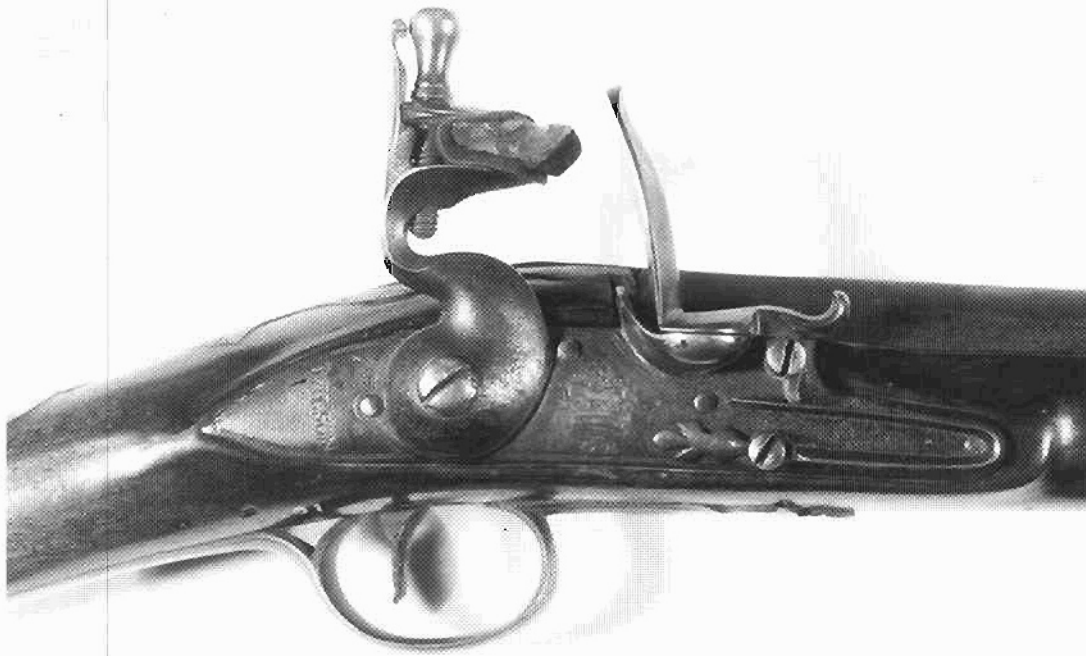
Figure 5. Slightly convex lock from a Brown Bess stocked Wilson Cypher gun. It is 6\frac{1}{8} " long and 1\frac{1}{16} " wide at the fence. Brass butt plate on Brown Bess stocked Wilson Cypher gun. The tang is 4" long.
