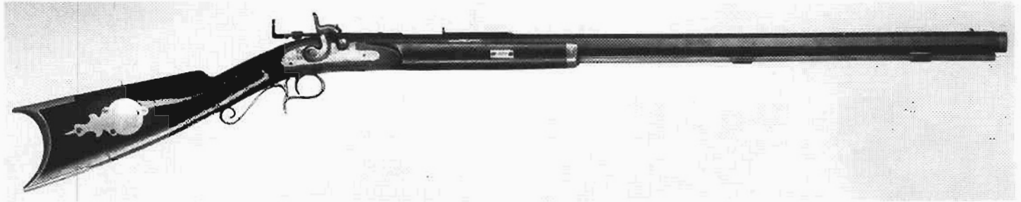
Figure 5. Characteristic half stock rifle by William Dixon of Adams, N.Y. The aperture rear sight is of unusual form, but otherwise the rifle is of a very common type; made in the 1860s, it is like hundreds of rifles made between about 1840 and 1870 in New York State. Photo: author.
