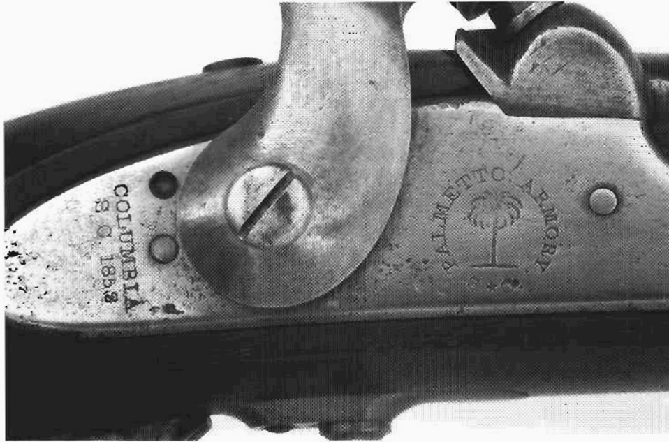
No. 2. Lockplate markings from a real Palmetto pistol. Note the circular base lines under the lettering in the semi-circle.
