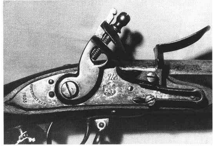
Figure 4. This 1805-dated lock has a curved, inclined "Springfield" behind the cock and the eagle's head is turned toward the muzzle. The frizzen spring finial is pointed and the frizzen's toe is straight.
