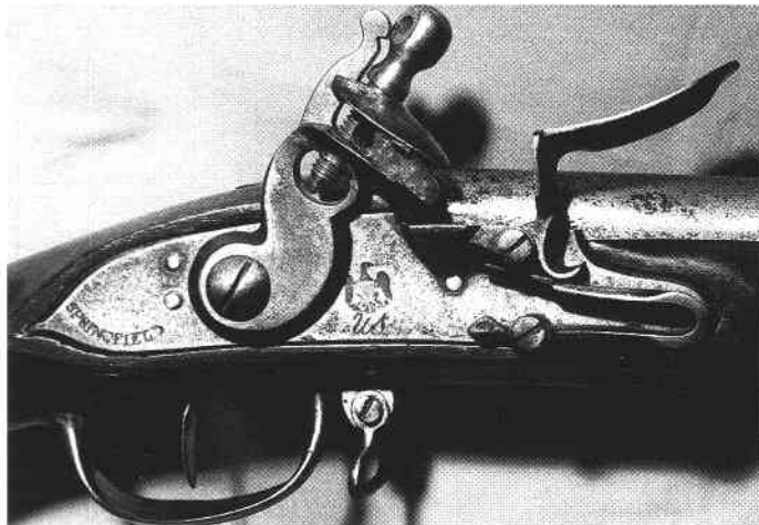
Figure 3. The lockplate markings of an 1803-dated Springfield musket. The eagle's head is turned toward the muzzle. The frizzen spring finial is pointed. The frizzen's toe and cock's top are curled.
