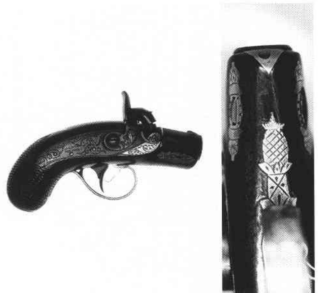
Figure 16. This is the piece which was made some time circa 1850-55 and has the last (5th) Deringer company legend. It is of the size everyone refers to as a "peanut." It is included here because it has two unique features. The butt is bag shaped and it has the shortest known barrel length, measuring 15/16 inches. It is .36 caliber.
