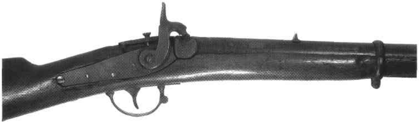
Figure 3. Billups & Hassell Texas Contract Rifle (second type)—depicting detail of backaction lock and bolster. Courtesy of George Wray, Jr.
