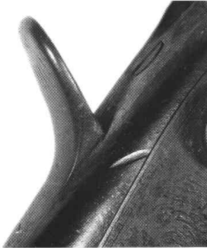
Figure 24. Close-up of the thumb piece for use with the sliding bayonet.
