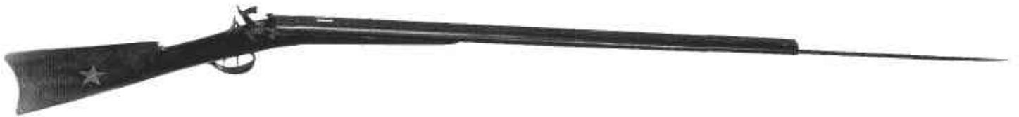
Figure 19. Over-all view of Green's double barrel rifle with the sliding bayonet partially extended. Hammers are at half cock.
