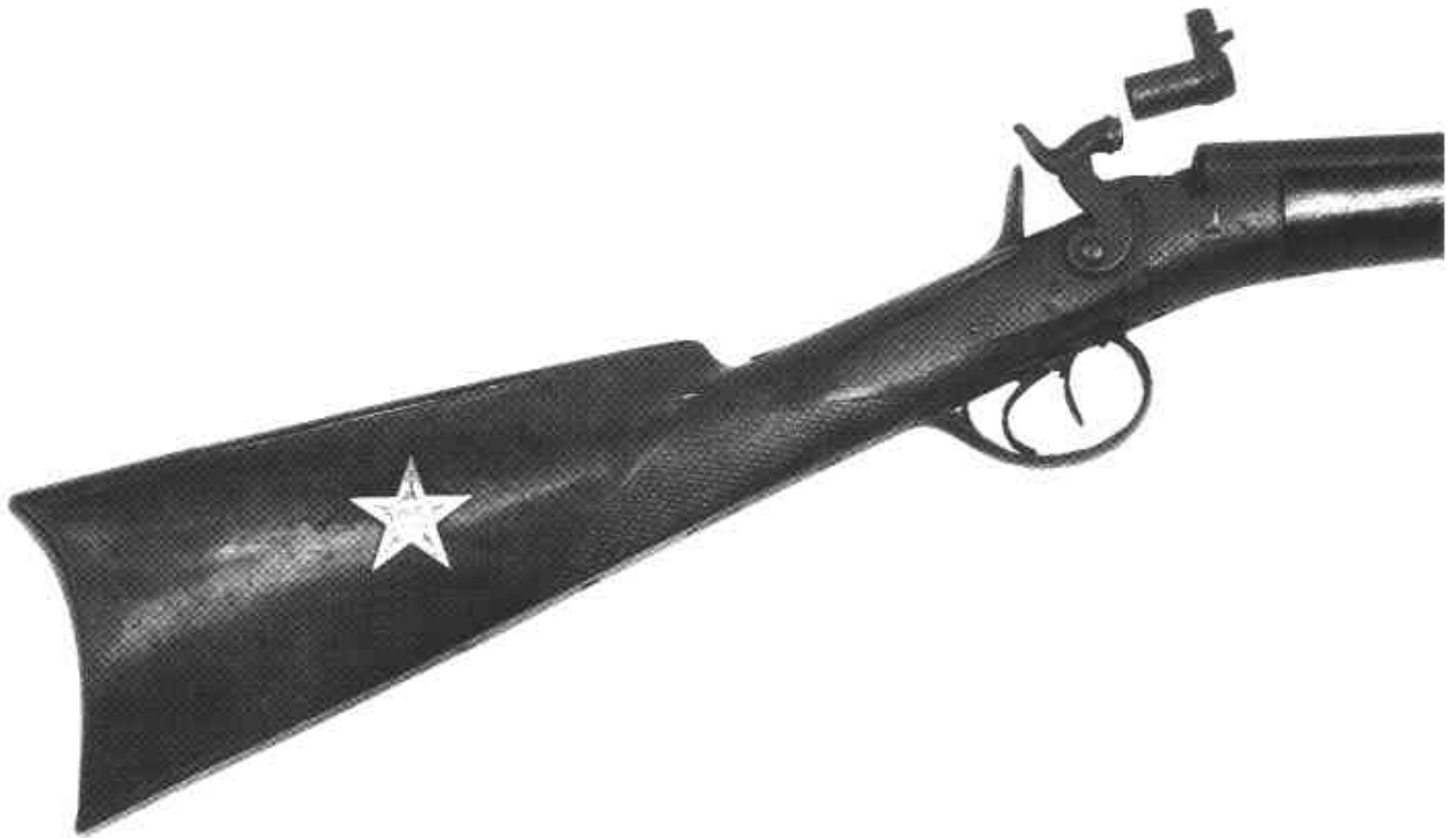
Figure 22. Close-up of right side of Green's rifle showing one of the cartridges removed and the thumb-piece.
