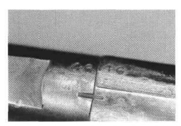
Figure 3. Bottom of barrel and receiver junction showing the register mark and matching serial numbers.
