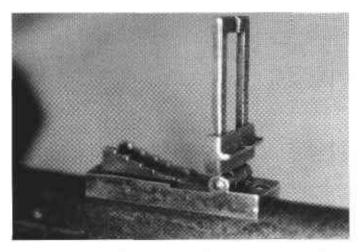
Figure 2. Top of barrel showing the Barnes-type rear sight.
