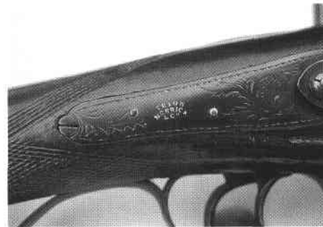
Figure 23. The stamped back-action locks.
