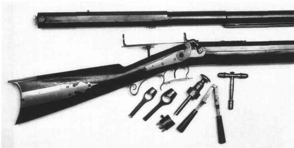
Figure 2. Heavy match rifle with extra barrel by Edwin Wesson (1811-1849) of Northboro, Massachusetts, ca. 1840-45. Accessories include false muzzle, bullet starter, bullet mold, patch cutters, and nipple wrench. (Courtesy of the late John Bicknell, Jr.)
