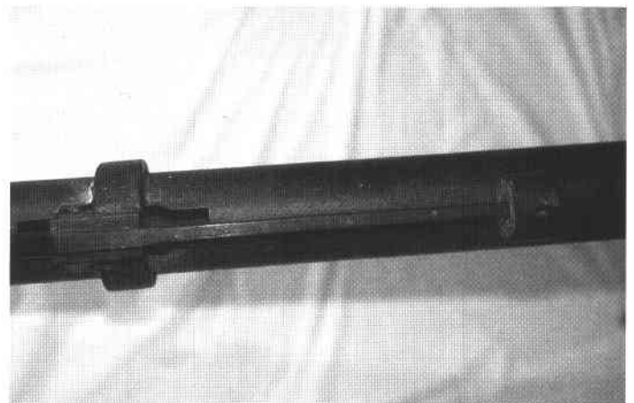
Figure 8. Restraining lever showing seconds of rocket burn time and the counterweight set on eight seconds. Author's photograph.
