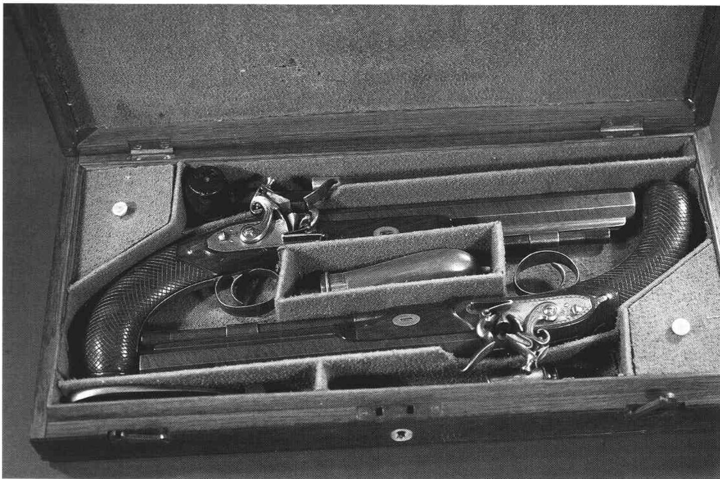
Figure 11. A cased pair of flintlock duelling pistols, c. 1810, by Thomas Manton, ex. Keith Neal collection and shown in plate 164 of The Mantons: Gunmakers . Marked "London" on the lockplates, they were probably manufactured in 1817. They feature French-style cocks and removable breeches marked "T. Manton/PATENT" in a poinçon. The barrels are marked on the underside with the serial number 10. Firearms by this maker are exceptionally rare; Neal & Back were able to catalog only nine examples (including just two sets of duellers) in their book and supplement.
