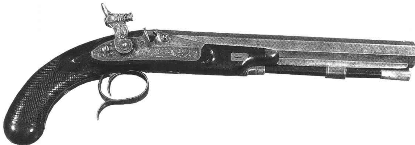
Figure 12. One of a pair of cased patchlock duellers, serial number 6756, by Samuel Nock. The detachable strikers are removed for recharging by lifting a thin lever on the side of the hammer, a system popularized by Joseph Manton. Extra strikers are supplied in a tin canister. The engraving on the lockplates is of the highest quality but is so delicate and understated that it is hard to see without holding the pistols up to the light. The 52-caliber, 10-inch barrels are marked on top "Samuel Nock Regent Circus" and have gold poincons at the breech. Nock did business at this address from 1823 until his death in 1851.
