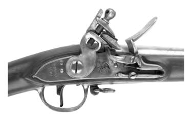
Figure 2. Typical lock markings on Henry manufactured musket.
