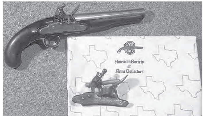
Figure 11. Prototype Brass Barreled Pistol with Screwless Lock, by H. Nock. Collection of P. S. Wainwright/once H. Blackmore's.
