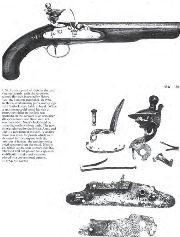
Figure 2. Patt. 1796 Cavalry Pistol of 2nd Dragoon Guards/dismantled Screwless Lock by H. Nock. Royal Armouries Collection/H. L. Blackmore, English Pistols, Arms & Armour Press, Lond. 1985.
