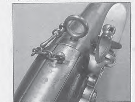
Figure 6- This view of the trigger guard shows where the pin penetrates the (just in front of the large-headed screw) It has an eccentric end which enables the flat spring safety to move laterally when the pin is twisted.
