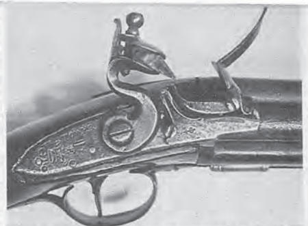
Enlarged photo of first model lock plate providing a better study of the odd Queen Anne Period frizzen spring, the moisture proof fitting of forward portion of lock plate to barrel group. The Tower Markings are uniform for this model, of which 500 were contracted for and delivered. A total of 635 first and second models were made by Henry Nock between the years of 1779 and 1788. Note the minute and uniform pitting on the barrel group of this particular gun, which can be considered to have been used at sea with this effect from salt air. (From the Harry H. Mann collection)
