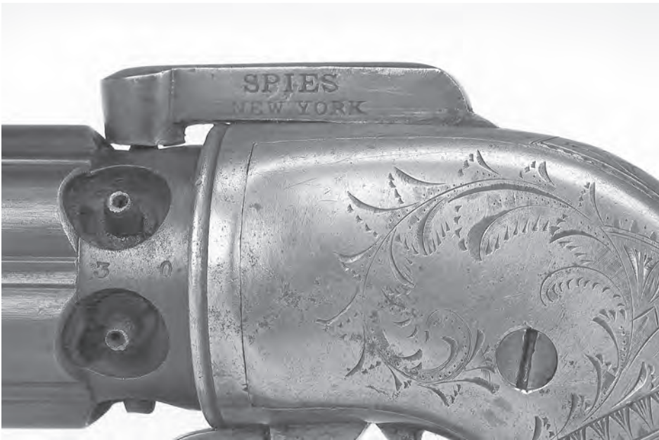
Figure 6. Detail showing the "A.W. Spies" marking, engraving style, removable nipples and production number on the Allen & Grafton Dragoon pepperbox.
