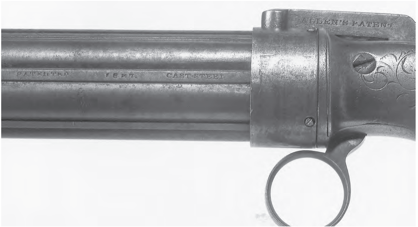
Figure 12. Detail showing markings, engraving, ring trigger and nipple shield of Allen Norwich pepperbox.
