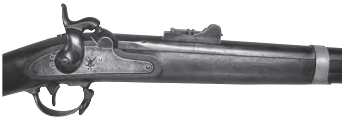
Figure 25. Model 1855 screwed-on long-range rear sight.
