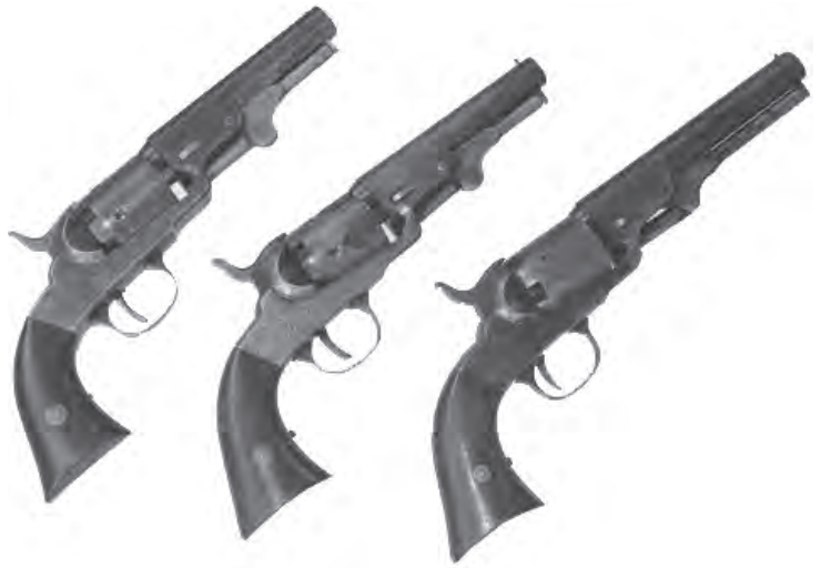
Figure 5. The evolution of the Bacon Manufacturing Company line. On the left, an octagonal barrel first model; in the middle, a fluted cylinder round barrel second model, and on the right, his final third version with an improved loading lever link.
