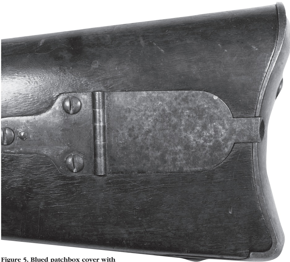
Figure 5. Blued patchbox cover with blued rounded head screws.
