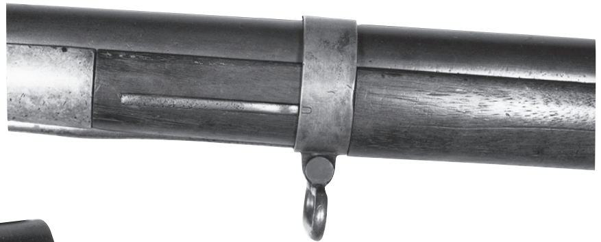
Figure 9A. Brass front barrel band with "U" stamping, and with sling swivel attached; band retaining spring and rear part of brass noscap also visible.
