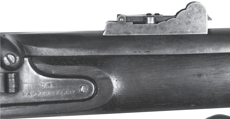
Figure 3A. Long-range rear sight and front part of lockplate with "U.S. Harper's Ferry" stamping.
