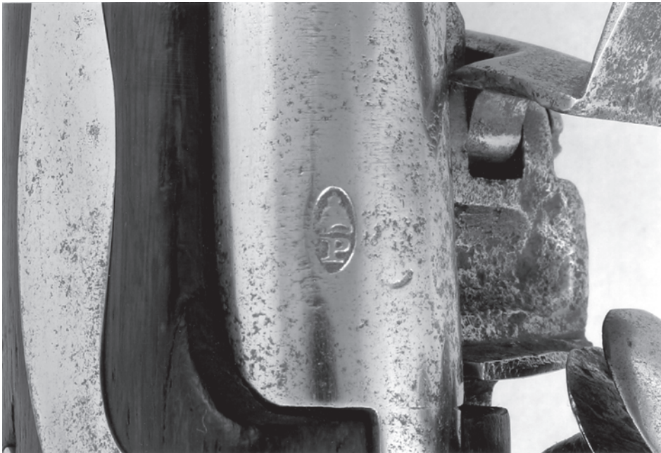
Figure 6. Liberty cap proof mark stamped into musket barrels passing proof test firing.
