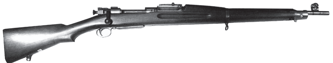
Hybrid M1903 rifle chambered in .303, made by Remington under contract to Great Britain. Remington R&D Facility collection.
