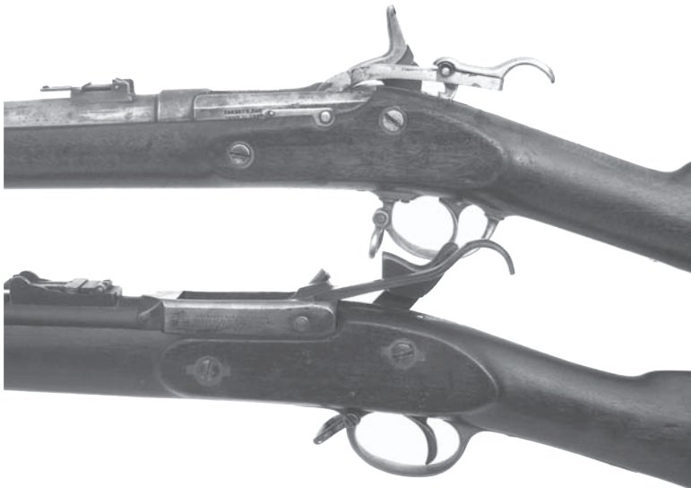
Plate 14. A reverse view from Plate 13. Note that the Roberts breech block is locked down by a spring-loaded latch, whereas the Peabody block is held closed by an internal spring (author's collection and photograph).
