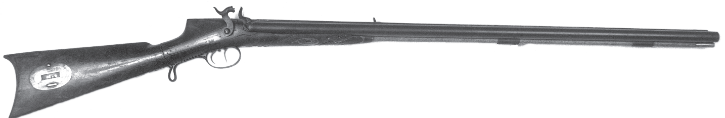
Figure 10. A Ben Mills rifle, typical in design and style of the guns he made in Harrodsburg. It is a double-barreled rifle of .43 caliber. Both locks are marked MILLS/HARRODSBURG/KY.
