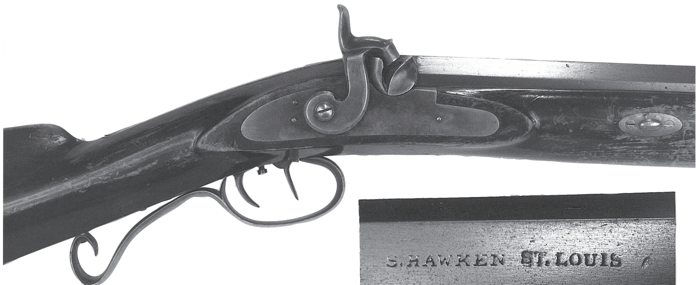
Figure 2. The breech-crest area of Carson's Hawken. The graceful curved scroll in the grip of the trigger guard is almost unique to Hawken plains rifles. INSET: The mark on the top of the barrel.
