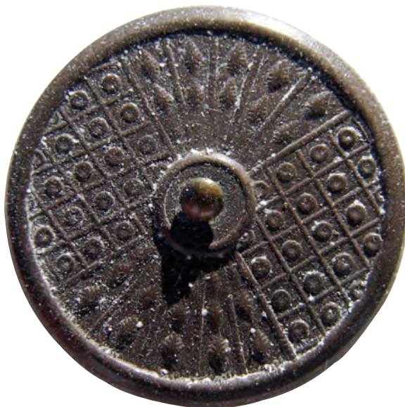
Figure 63. The little white speckles on this hard rubber button are "sulfur bloom", the result of too much sulfur in the formula. The speckles of sulfur wipe off and are not harmful.
