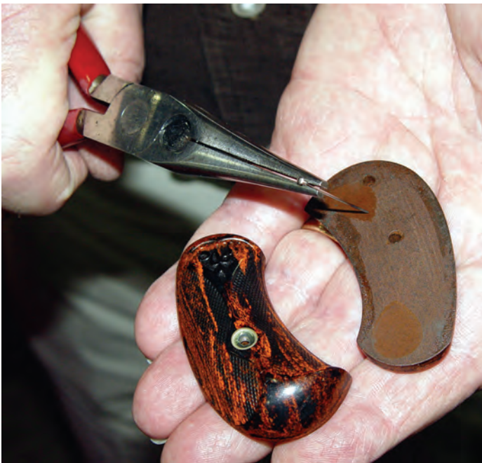
Figure 26. The hot needle should be applied in a hidden area to avoid surface damage.
