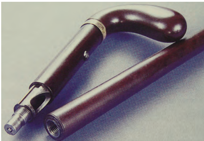
Figure 13. 9. Remington covered the shafts of many of their cane rifles with gutta-percha which provided a handsome appearance and endured both use and abuse. Elliott Burka collection.
