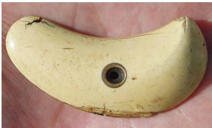
Figure 73. Remington Smoot Celluloid grip with typical shrinkage cracks. Jim Shaffer collection.
