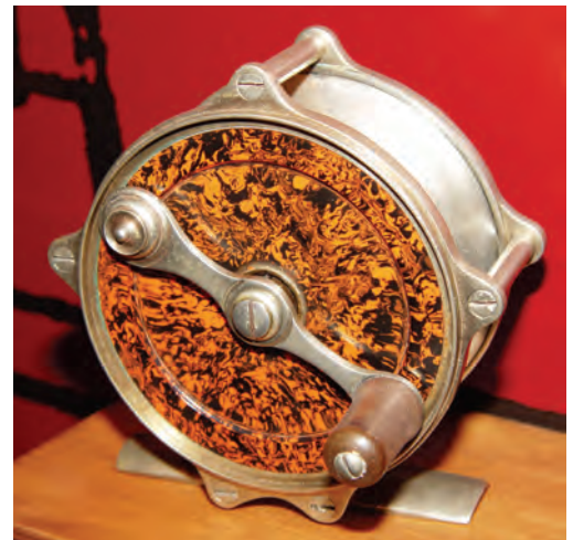
Figure 21. The beautiful red mottled side plates of circa 1877 Philbrook and Paine fly reels are often declared to be “hard rubber,” but in fact, they are molded of “Mud.” Image courtesy of American Museum of Fly Fishing.
