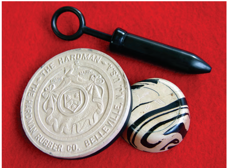
Figure 50. Not all hard rubber was black, although carbon black was a reinforcing filler. Mottled red hard rubber is frequently encountered, but lighter colors, although available, never proved popular in firearms.
