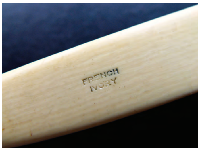
Figure 70. A Celluloid knife handle with laminations to imitate the look of genuine ivory, here marked “French Ivory.”
