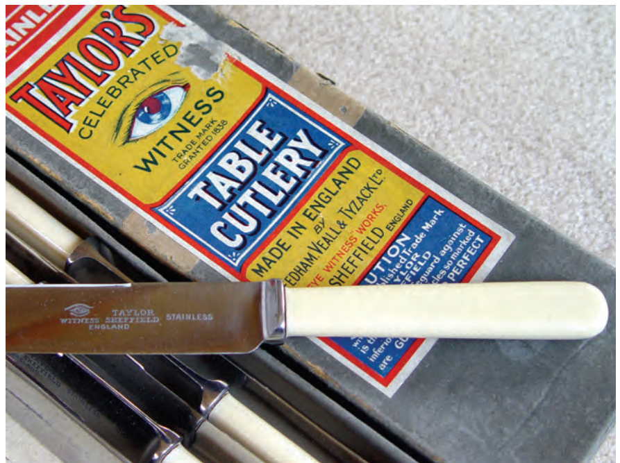
Figure 65. Celluloid (cellulose nitrate) and later cellulose acetate found widespread acceptance for use in knife handles.
