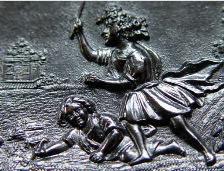
Figure 18. The surface detail of products molded from “Mud” was excellent; this is the surface of a Littlefield & Parsons picture frame.
