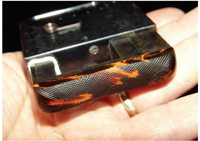
Figure 58. Mitrailieuse mottled red and black hard rubber cover with checkering molded in.
