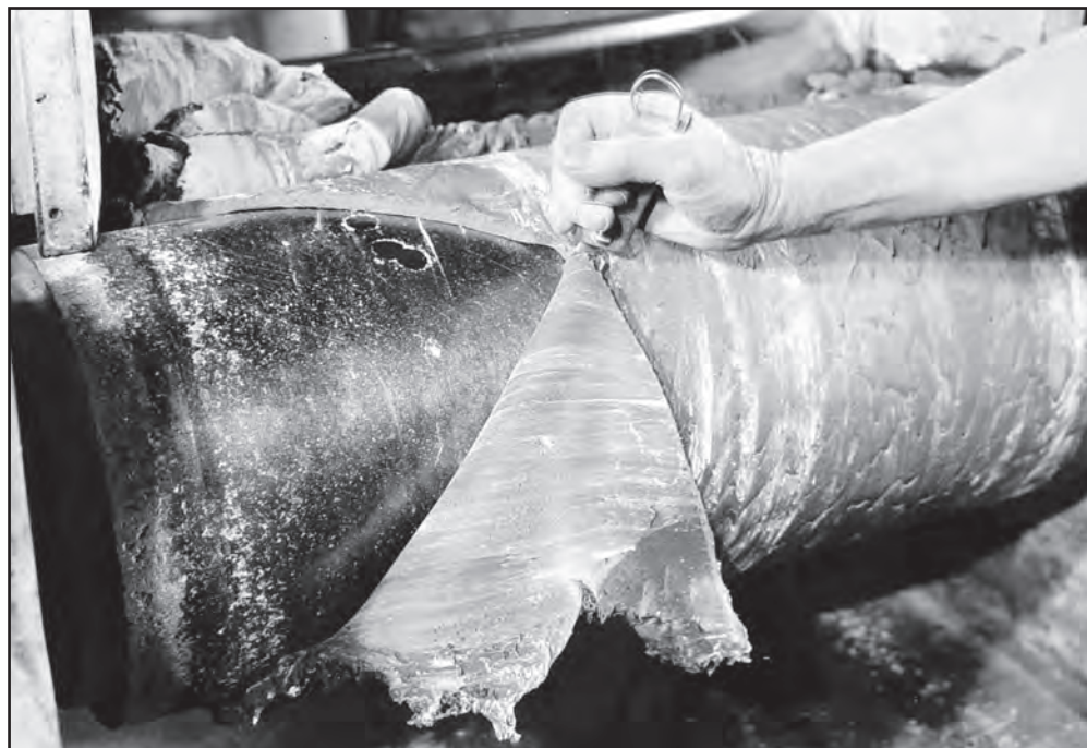
Figure 29. A two-roll mill used to mix sulfur and compounding ingredients with raw rubber “in the solid.” The hardness of the vulcanized rubber varies with sulfur concentration.
