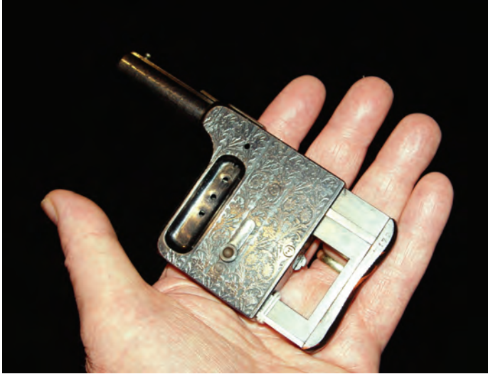
Figure 57. A French Mitrailieuse palm pistol with a hard rubber operating rod cover.
