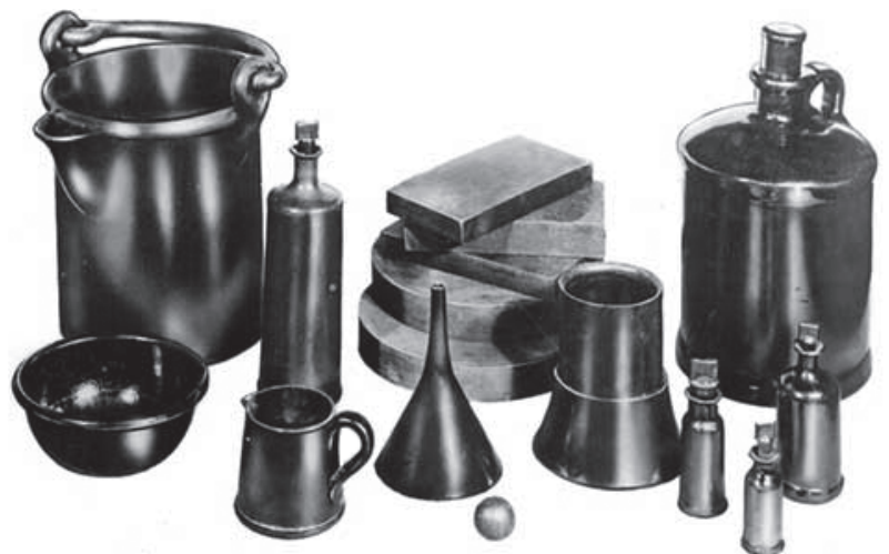
Figure 3. Typical products made from gutta-percha during the 1850s and 1860s. Note the natural satin finish. Gutta-percha offered wonderful resistance to bio-degradation.
