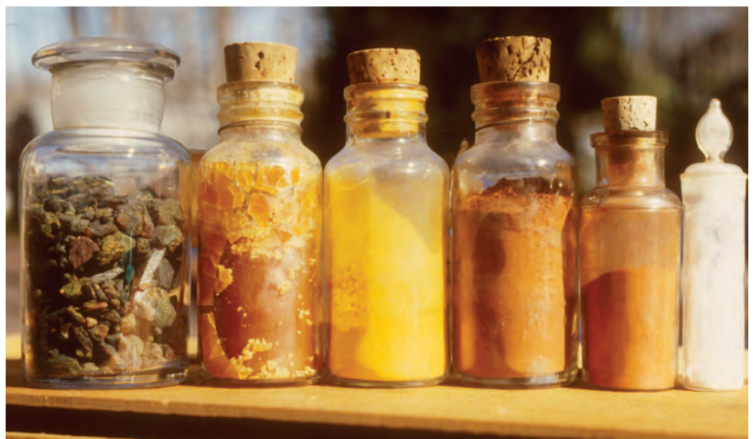
Figure 17. "Mud" was a mixture of hot-melt resins similar to rosin or shellac used in molding. Hardness was adjusted by the choice of resins and diluents; pigments offered a broad range of colors.
