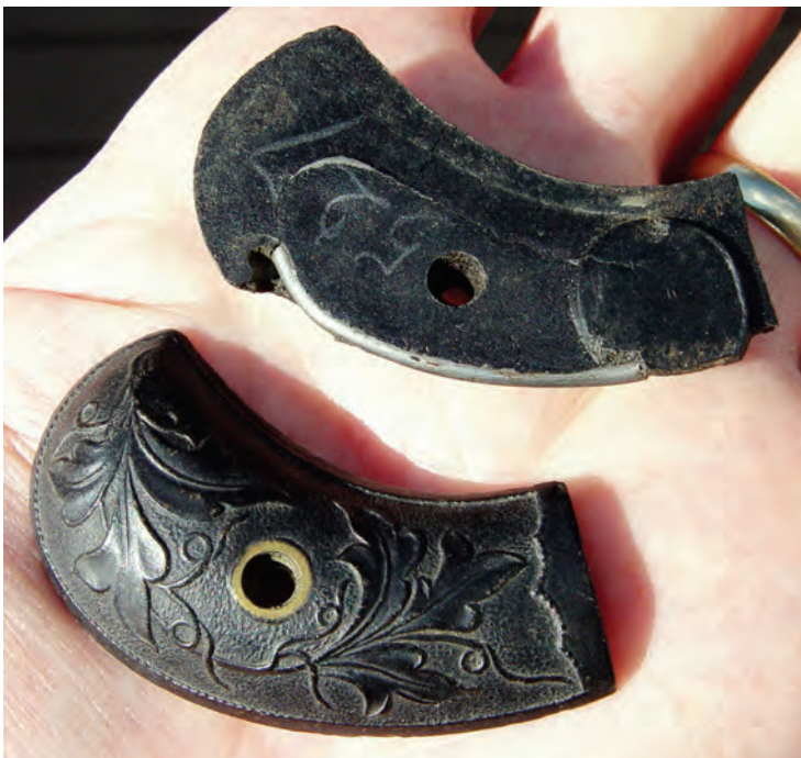
Figure 23. These S&W presentation cases were molded by the Littlefield & Parsons Company from a mixture of shellac and wood flour.
