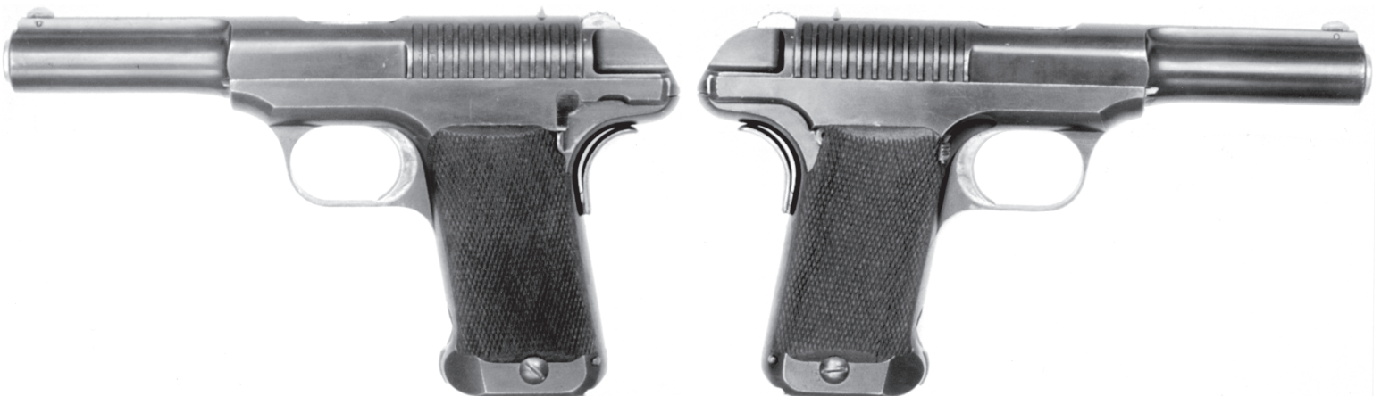
Figures 6 and 7. Left and right views of the original Savage Model 1907-10, .45 caliber test pistol, Serial #1, that was used for the prototype for the redesigned Model 1910 test pistols.
