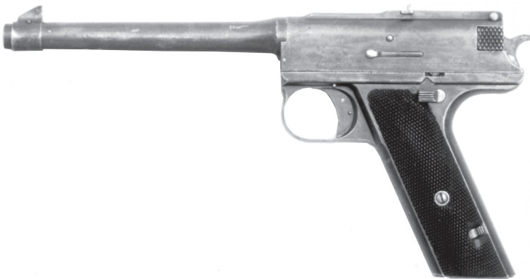
Figure 10. Left view of .45 caliber pistol (Serial #1), supplied by Grant Hammond for the January 1907 trials. This design was rejected because the magazine automatically ejected when the cartridges were spent. It later became the basis for the successful High Standard .22 caliber pistol.
