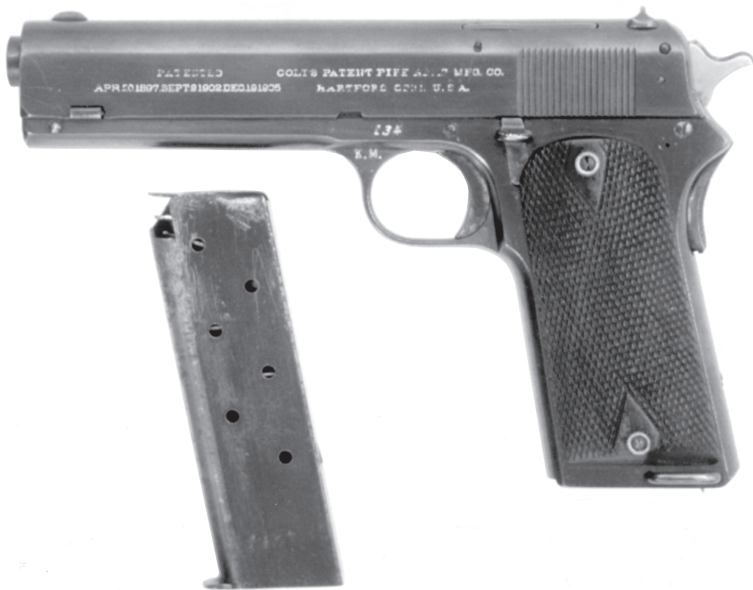
Figure 8. Left view (plus magazine) of the Colt, .45 caliber pistol (one of 200), supplied for the January 1907 military trials, the predecessor of the famous Colt Model 1911 automatic service pistol. The pistol is Serial #134.
