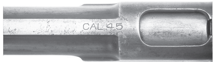
Figure 17. Factory legend on a refurbished Savage .45 caliber pistol sold prior to WWI. These pistols have all the slide legend lettering removed from the top of the slide except for “CAL.45”.
