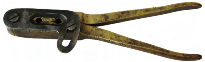
Figure 10. Standard Ames (unmarked) two cavity bullet mould (author's collection).
