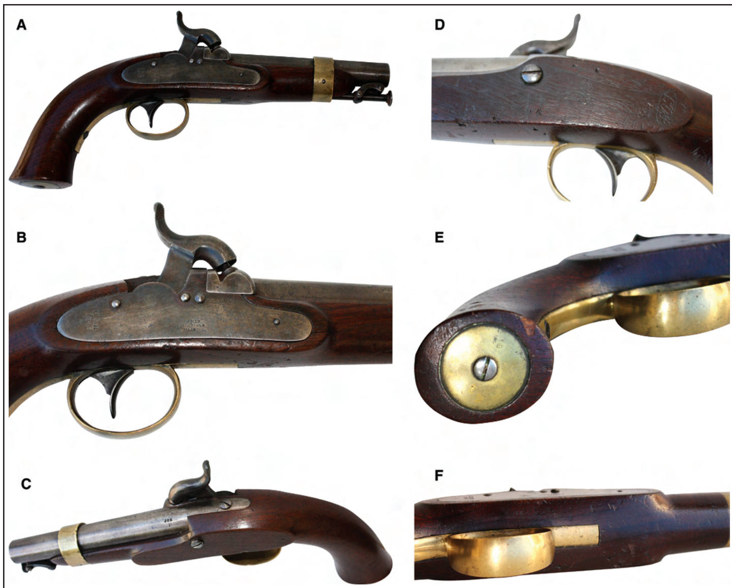
Figures 5 A, B, C, D, E & F. USR Boxlock Pistol (author's collection). Flayderman 6A-047.
