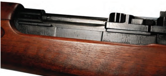
Figure 8. The segmented dovetail slot on the left receiver of a Venezuelan Contract rifle. Note the lower half of the slot is obscured by the stock.
