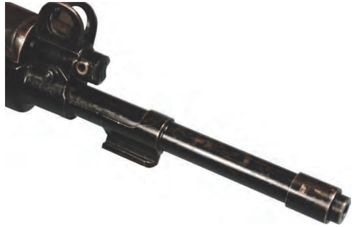
Figure 5. The collar-style muzzle cap used on all FN-49 contracts except Venezuelan and Egyptian. Note: the muzzle cap does not extend all the way to the muzzle; and the bayonet mount and gas regulator.
