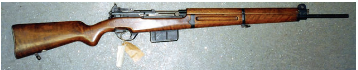
Figure 16. FN "D" Model, gas operated prototype rifle, Mid-Fall, 1946, Imperial War Museum photo.
