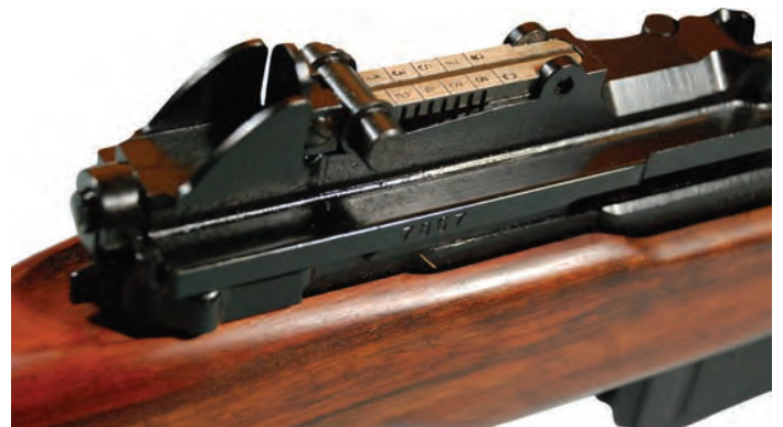
Figure 2. Receiver cover and rear sight of a Venezuelan Contract FN-49. Note the early style receiver cover lock at the rear of the receiver.
