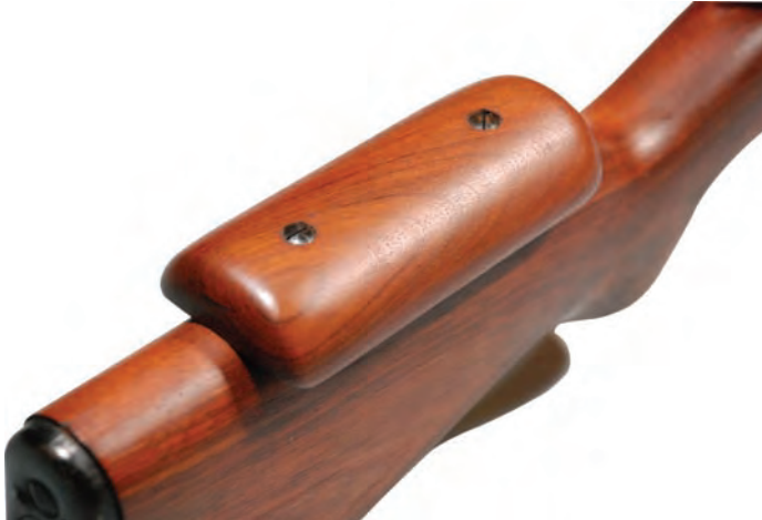
Figure 21. The ambidextrous cheek rest as seen on Belgian and Luxembourg sniper rifles.
