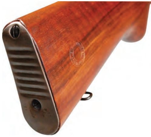
Figure 3. Corrugated steel buttplate in-the-white as used on Venezuelan, Columbian and Indonesian FN-49s. Note the Venezuelan Army cartouche on the buttstock of this Venezuelan Contract rifle.
