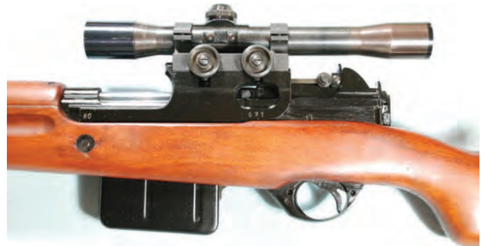
Figure 22. Close up of the base, ECHO mount and OIP scope of a Luxembourg contract sniper rifle.
