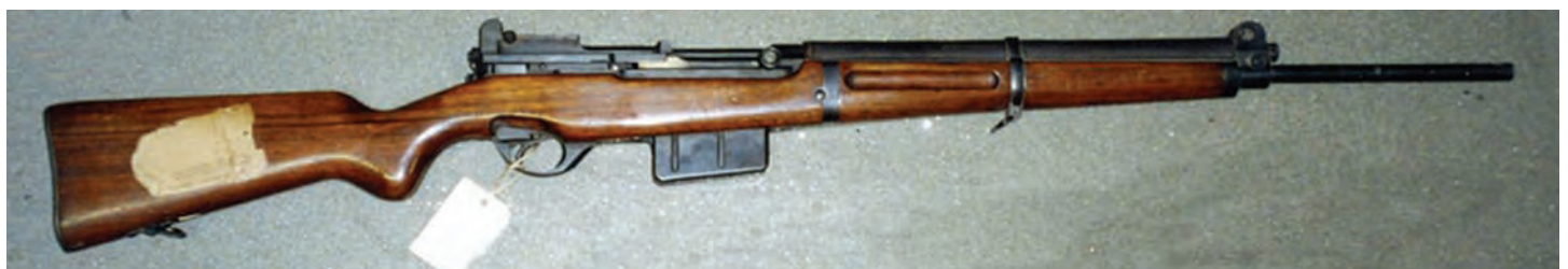
Figure 15. FN "C" Model, gas operated prototype rifle, Mid-Fall, 1946, Imperial War Museum photo.
