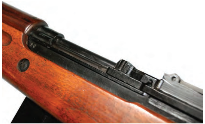
Figure 9. The full-length dovetail slot (lower half obscured by the stock). Note the recoil bolt on this late production Luxembourg FN-49.
