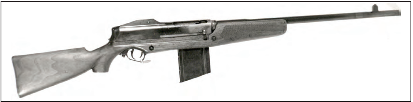
Figure 2. Primer-actuated rifle designed by Garand for National Bureau of Standards, 1919.
