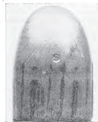
Plate 18. .45 automatic pistol bullet of U. S. Cartridge Company make without cannellure, fired through Thompson gun.
