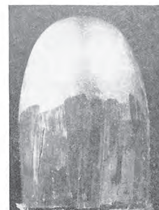
Plate 20. .45 automatic pistol bullet fired through .45 Smith and Wesson revolver.
