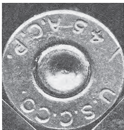
Plate 15. Firing pin imprint with elevation at base of crater, left on shell fired in 2nd Thompson gun.
