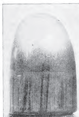
Plate 19. .45 automatic pistol bullet fired through Savage automatic pistol.
