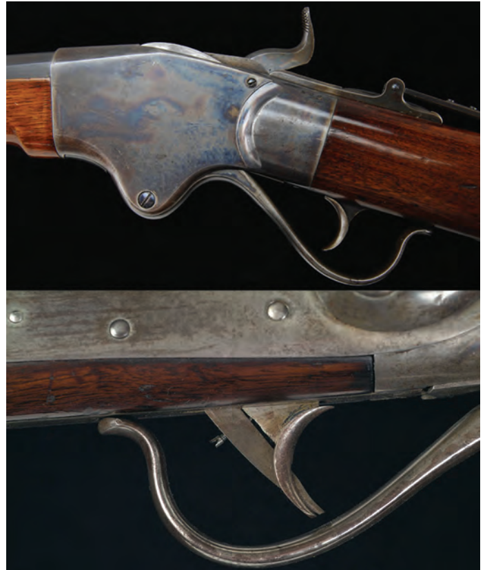
Figure 39. Standard trigger (top) set trigger (bottom).
