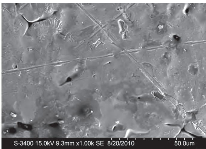
Figure 50. SEM analysis of an early model: 99% tin (Sn), 1% copper (Cu).
