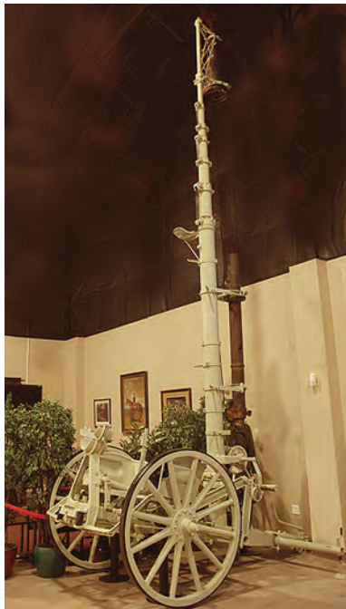
WWI German Mast Periscope used for artillery observation.
