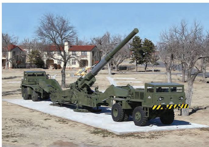
M65 240mm Gun "Atomic Annie" with its two heavy lifting trucks.
