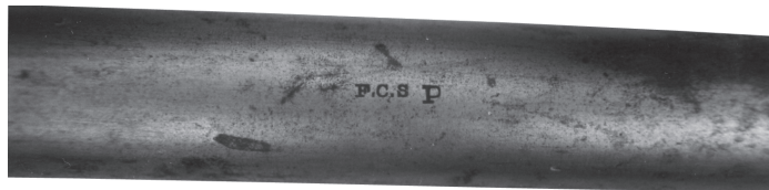
Figure 15. Underside of barrel proof inspector's markings (F.C.S.) seen on 1864 muskets. (Author's Collection)
