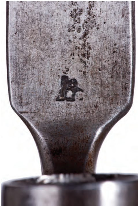
Figure 19. Close up view of cipher stamped base of blade. Note hairline imperfections evident on blade.
