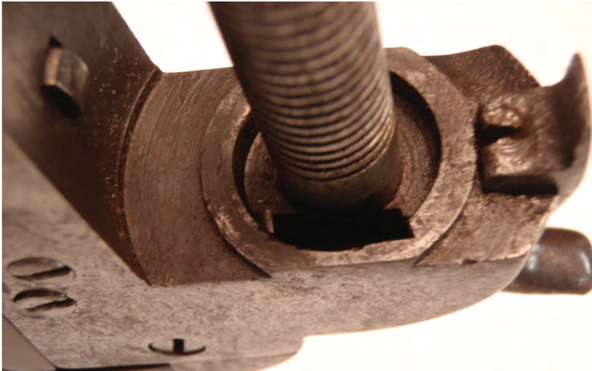
Figure 20. Pawl cut on a Dance pistol.
