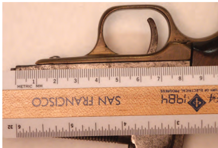
Figure 19. A Dance frame measuring 84 mm.
