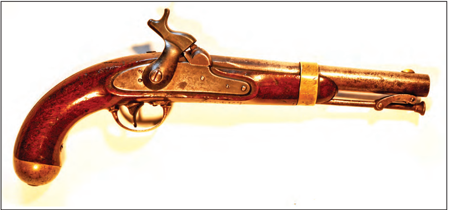
Figure 8. An unknown system with a disc primer device built into the hammer—perhaps a version of the Rupertus system shown in Figure 6.
