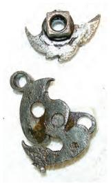
Figure 5. A close-up view of the tumbler and the two-piece bridle.
