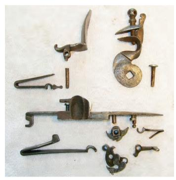
Figure 4. An disassembled view of the lock clearly illustrates the elongated cock screw which passes though the tumbler.
