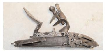
Figure 3. The interior of the lock shows the absence of screws with all parts being hooked into place with pins. The two-piece tumbler bridle can be seen which is rotated into position and held in place by the cock screw which passes through the tumbler and the peg for the sear.
