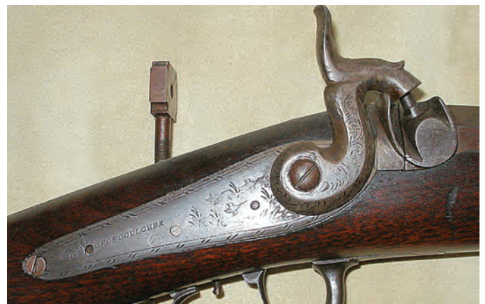
Figure 17 C. Back action lock.
