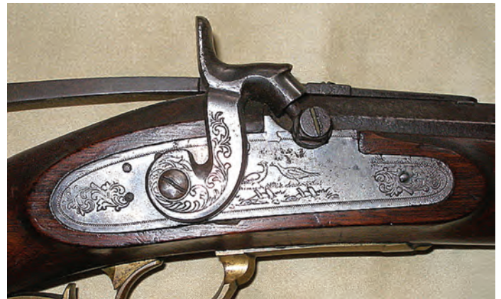
Figure 17 B. Front action lock.
