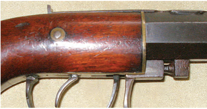
Figure 17 D. Slide lock.
