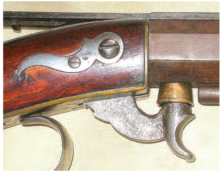
Figure 17 A. Underhammer lock.
