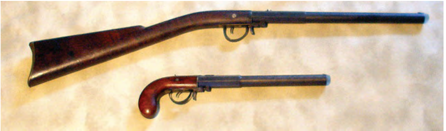
Figure 36. Michael Carleton, Haverhill. Slide bar underhammer rifles and pistols, c. 1845. His underhammer arms featured a unique slide hammer percussion ignition system.
