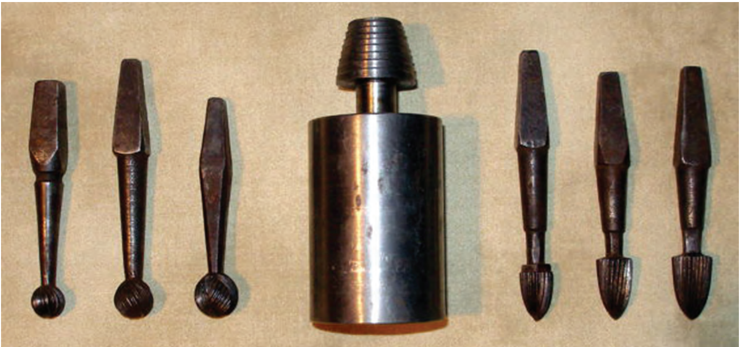
Figure 29. Mold cherries and bullet swage.
