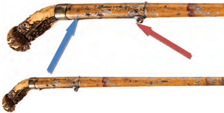
Figure 9. Two views of a cane gun marked "FAIRBANKS PATENT BOSTON." The collar and tip of the gun are made of brass. The simple undercock percussion lock is to similar cane guns made in this country and in England starting in the mid-1820s. The hammer (red arrow) has a hole for a line or ring to facilitate cocking the gun. The trigger (blue arrow) is in its closed and concealed position. The stag grip and faux bamboo painted barrel were popular designs with many makers of cane guns. (Photos courtesy of Matt Parise, Rock Island Auctions.)
