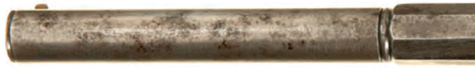
Figure 13. A Fairbanks belt or holster pistol with a 7-inch barrel. The barrel is part round, part octagonal, with a one piece hammer/trigger identical to the pocket model. This example is stamped with serial number 19 under the barrel and the frame. Note the two screws that hold the grip in place. The barrel is die stamped "FAIRBANKS, BOSTON," and "CAST STEEL" on the octagonal portion of the barrel. Other than the shape of the grip, the design and finish of the belt pistols is identical to the pocket models. (Collection of Perry Hansen, photo courtesy Rock Island Auctions.)
